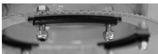
When the chute is assembled it should rotate easily without any friction. If not, check whether the plates are fastened too tight. Ensure that the different types of plates are in the right sequence. See picture above. The auger screw can be adjusted to move it in or out for screw engagement. If turning the chute handle cause the screw to jump over the chute teeth move the auger screw in by unloosing the support bracket screw and pushing it in.
